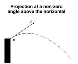
If the projectile is launched with an initial speed u at angle  $\theta$  above the horizontal, its initial horizontal component of velocity =  $u \cos\theta$ . Because its horizontal component of acceleration is zero, then its horizontal component of velocity is constant. Hence the horizontal component of its displacement from launch, at time *t* after being launched,  $x = ut \cos\theta$  and its initial vertical component of velocity =  $u \sin\theta$ . Hence:
