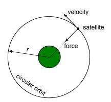
Hence  $v^2 = G M / r$  gives the speed of a satellite in a circular orbit.
