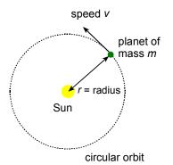
A planet moving round a circular orbit or radius *r* in time *T* has speed
