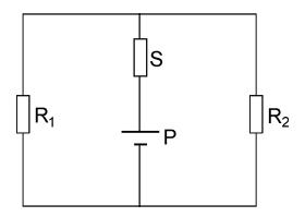
where the cell P represents the primary coil which is producing the flux, much as a cell produces current in an electrical circuit, the resistor S represents the secondary coil, and the two resistors  $R_1$  and  $R_2$  are the side-arms of the transformer core.
