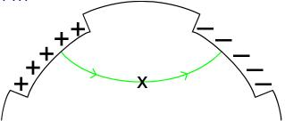
(c)(ii) The electric field exerts a force on the electric charge (in this case towards the + and away from the –), thus causing the rotor to rotate (anticlockwise).
