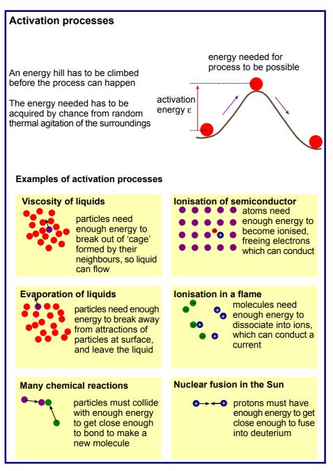
An activation process is one in which the particles have to overcome an energy barrier before the reaction or change can occur.
