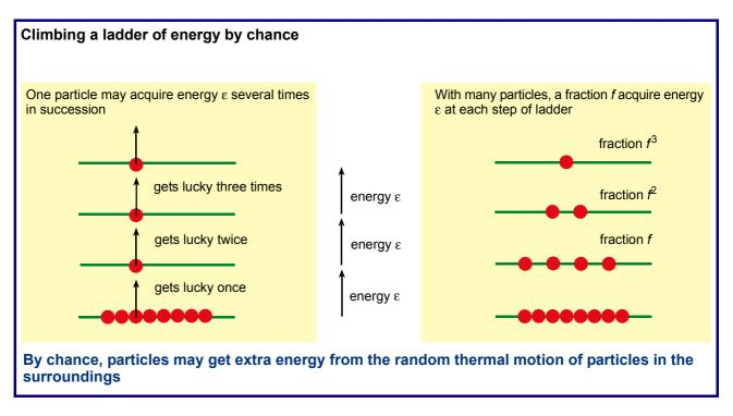
This diagram shows why only a small fraction of particles acquire energy much larger than average, through random collisions.
