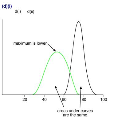
For the average force to be lower the maximum force must be lower. The head meets the air bag earlier than it would have hit the steering wheel, so the force starts to rise earlier.
